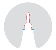
Designed to work with majority of Frame Cramps and Type 1 Ties, the Keyfix Non-combustible Insulation Retaining Disc (NCRD) has a unique patented spring loaded action, which clamps the NCRD to the main body of the wall tie.
